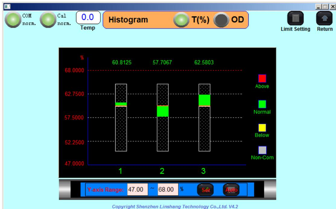
As shown above: rectangular box shows the upper and lower limits, and the filled chart shows the measured values.
